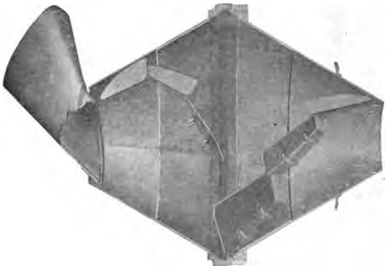
Fig. 11. Cross Section of Drum (front half cut away), Showing Blades and Lining.
